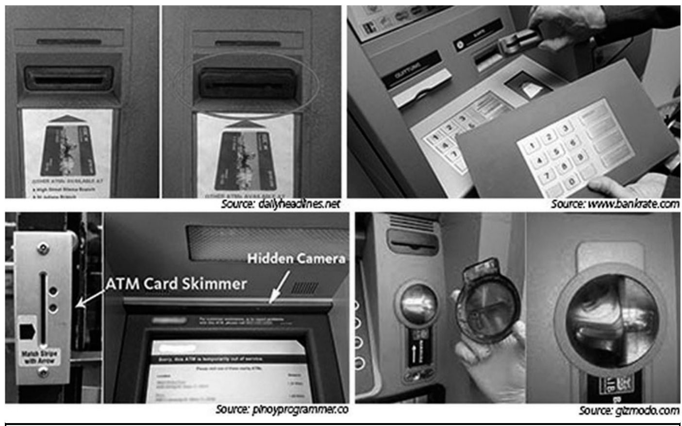
Figure 20-6 Skimmers attached to ATMs
