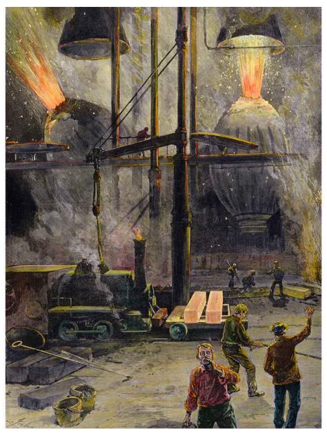
**The Bessemer process**, devised by the English engineer of the same name to convert iron into steel, improved the efficiency of all industries – from transport to the military.
