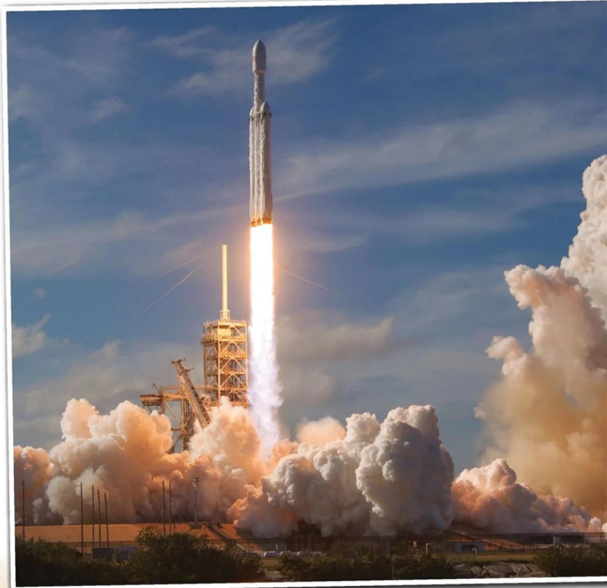
Right: SpaceX's huge Falcon Heavy rocket has a first-stage 'core' Falcon 9 rocket flanked by two identical Falcon 9s that act as boosters during launch
